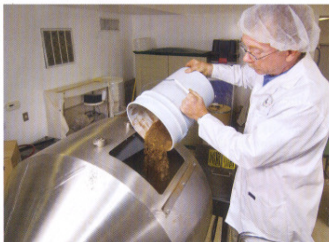
Munson says its mixer is suited for blending small quantities of additives as it inter-mixes ingredients – even trace amounts – thoroughly and rapidly.
