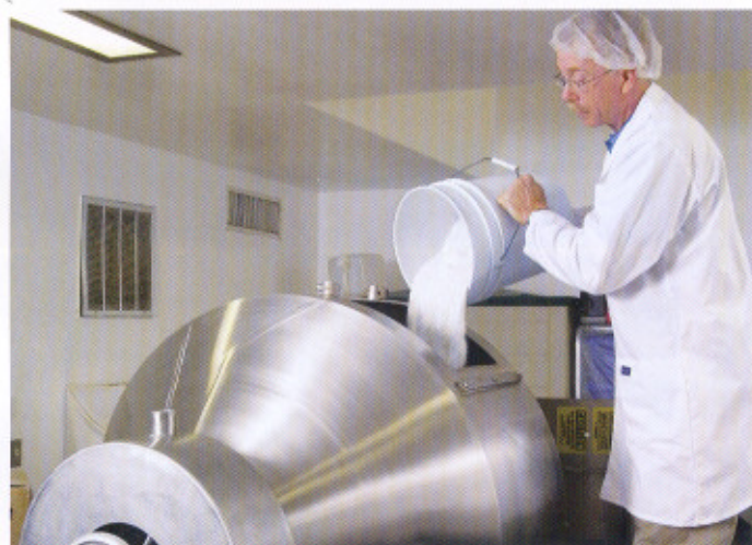
Munson says its mixer is suited for blending small quantities of additives as it inter-mixes ingredients – even trace amounts – thoroughly and rapidly.
