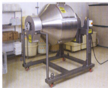
The 0.28m 3 capacity Munson Rotary Batch Mixer at Daily Manufacturing's plant. The drum rotating on external twin pillow block roller bearing assemblies gently but thoroughly mixes ingredients having different bulk densities, according to the manufacturer.
