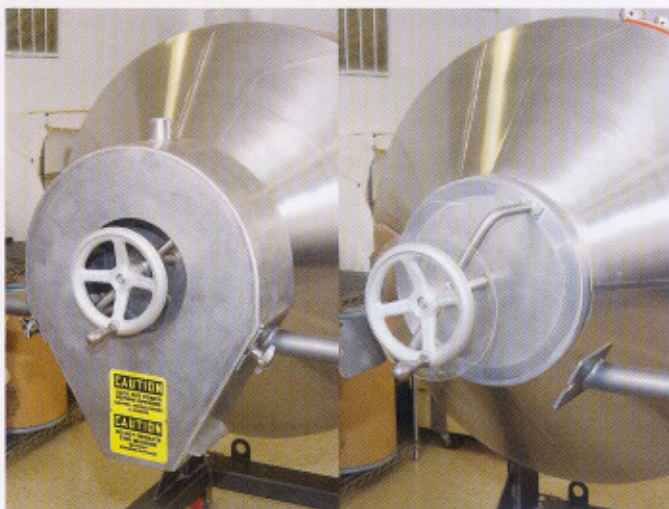
Continuous rotation of the drum helps assure total discharge, which is important as Daily Manufacturing changes products processed in the mixer several times a week. Hand wheel eases operation of the discharge gate.
