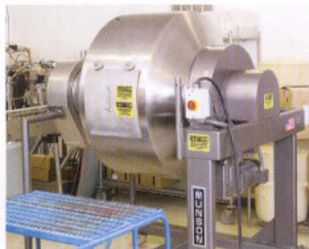
The 0.28m 3 capacity Munson Rotary Batch Mixer at Daily Manufacturing's plant. The drum rotating on external twin pillow block roller bearing assemblies gently but thoroughly mixes ingredients having different bulk densities, according to the manufacturer.
