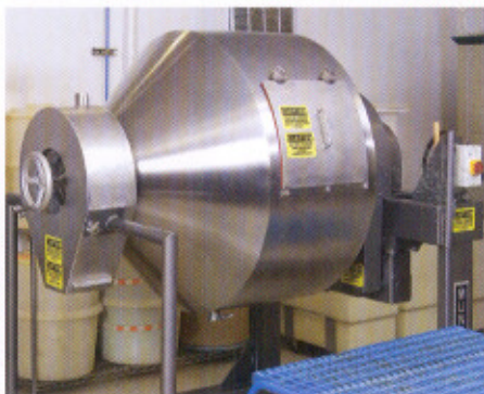
The 0.28m 3 capacity Munson Rotary Batch Mixer at Daily Manufacturing's plant. The drum rotating on external twin pillow block roller bearing assemblies gently but thoroughly mixes ingredients having different bulk densities, according to the manufacturer.
